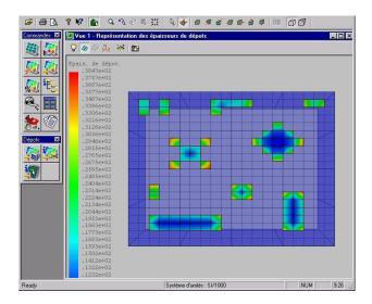
The graphic here is a simulation plating model of one of the problem boards with one major difference: the darker blue border is the model of a simple shield around the perimeter of the board.
