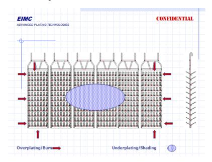
A little trial and error by imposing simple shields or barriers can fix a situation like the one above. All the available plating current still goes into the cell, it's simply redirected. "Shading" begins to go away.
